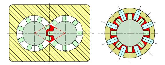
Figure 7, Intermeshing region in twin screw extruder (left) and in VIP mixer (right)
