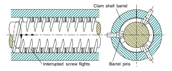
Figure 3, Schematic of the Buss Kneader
