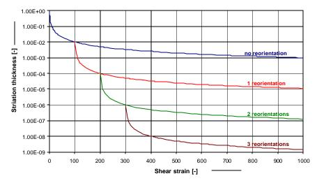
Figure 2, Striation thickness versus shear strain with reorientation
