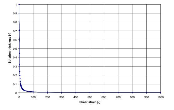
Figure 1, Striation thickness versus shear strain
